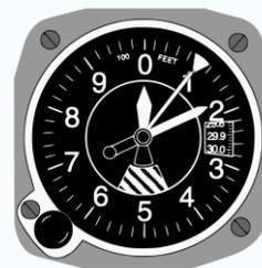
On a sensitive altimeter, the sea level reference pressure can be adjusted by a setting knob. The reference pressure, in inches of mercury in Canada and the US and millibars (or hectopascals) elsewhere, is displayed in the *Kollsman Window*, visible at the right side of the aircraft altimeter shown here. This is necessary, since sea level reference atmospheric pressure varies with temperature and the movement of pressure systems in the atmosphere.
