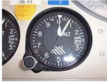
Kollsman-type barometric aircraft altimeter as used in North America displaying an altitude of 80 feet.
