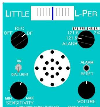
Since the device relies on internal crystal oscillators for receiving frequencies, the device cannot be configured from its factory preset frequencies. These frequencies typically include the emergency frequency of 121.5 MHz, the training frequency of 121.775 MHz, and the military and civilian emergency frequency of 243 MHz. Some older L-Pers may also include 121.6 MHz, an older frequency formerly used for training.
