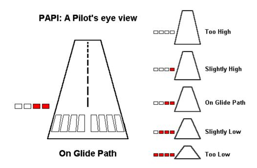
A PAPI is a system of lights that provide visual descent guidance information during the approach to a runway. This system provides a visual glide path that allows for safe obstruction clearance from the start of descent to the threshold.
