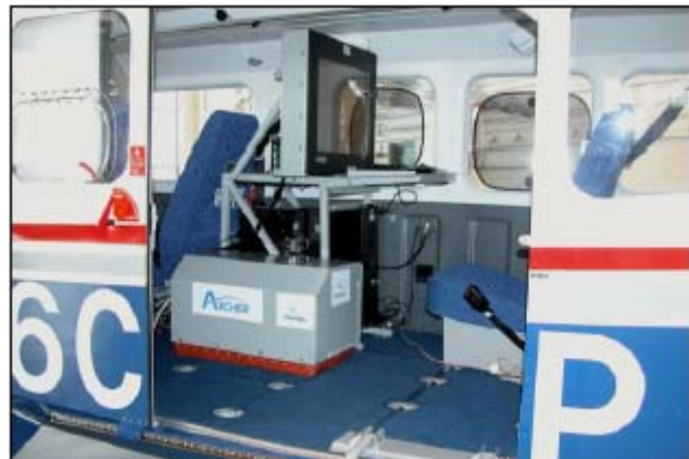
ARCHER system installed with custom-designed rack and protective hood in the Gippssland GA-8 Airvan
