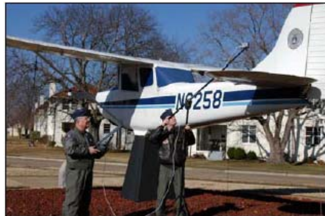
HSI operators collect the spectral signature of an aircraft on static display outside the CAP National Headquarters building at Maxwell AFB, Ala. The signature is then entered into the ARCHER airborne system and used in a test to determine if the HIS equipment will pinpoint the static display plane from the air.
